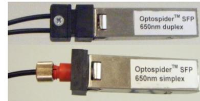
*Fig 2: Optospider™ SFP modules from Diemount. Above, the duplex model using two different fibers. Below, module designed for simplex transmission over just one fiber. Both modules work with visible 650nm sources.*
