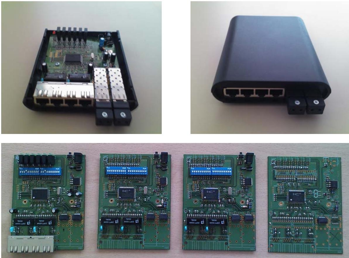
*Fig 4: The top images show the final design of the switch which is inside the black box. The bottom picture shows different PCBs in different stages of production.*
